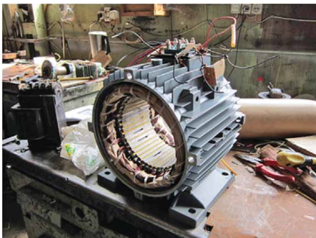
4 pav. Eksperimentinio šešiafazio variklio statorius Fig. 4. Stator of experimental six-phase motor
