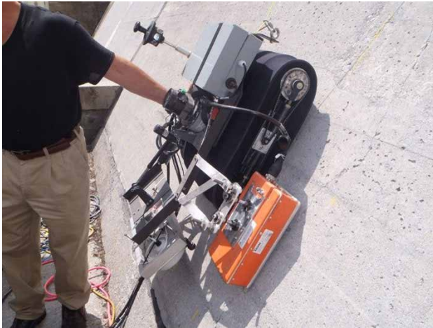
Figure 8. Experimental robot crawler used for NDE of Claytor dam
