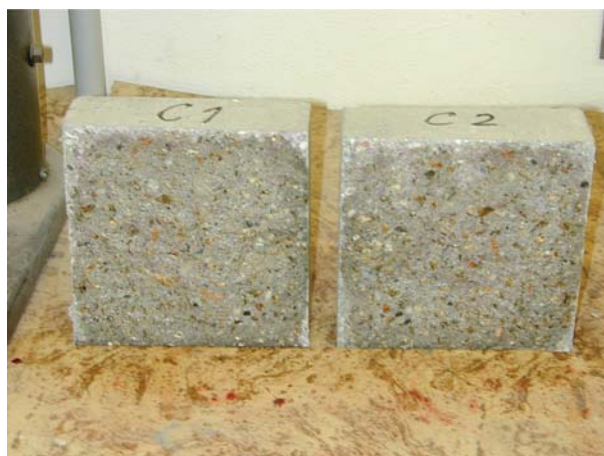
Fig. 1. Sample of formulation C placed in 98% CO 2 for 365 days, carbonation depth 75 mm, real sectional dimensions of sample: 150×150 mm (Scale: 1:5)
