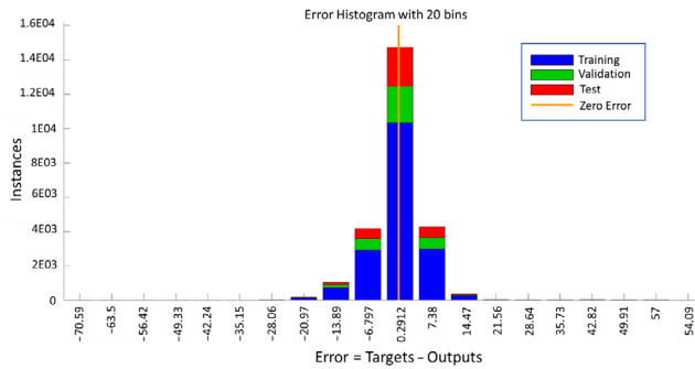
Figure 5. Error Histogram with 20 bins for 50-layer size neural network Scaled Conjugate Gradient
